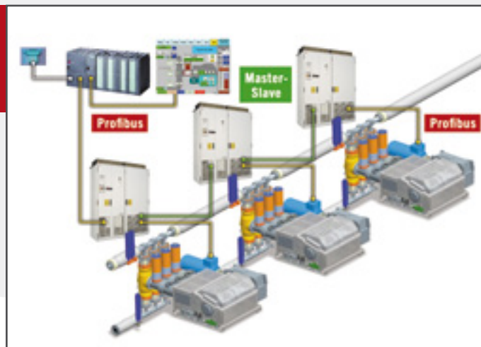
Three triplex sets of FELUWA MULTISAFE pumps discharging into a common main. FELUWA pump synchronisation controls phase shift and eliminates excitation of resonances significantly.
